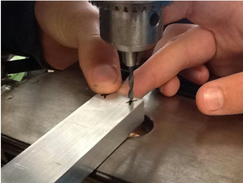
drilling holes for the hinges
