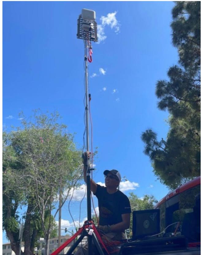
**Figure 4: Improved Drive-Testing Rig**
